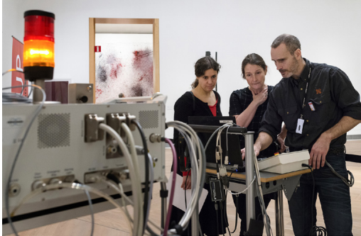
Figure 5. My Bundgaard, Thérèse Lilliegren and Kaj Thuresson performing XRF analysis of Rauschenberg's Monogram , 2016 (photo: Åsa Lundén/Moderna Museet)
