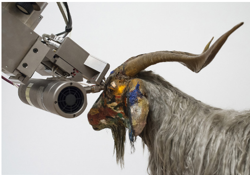
Figure 1. XRF measurements of elements in the paint layers. Robert Rauschenberg, Monogram (1955–59). © Robert Rauschenberg/Untitled Press, Inc./Bildupphovsrätt 2016 (photo: Åsa Lundén/Moderna Museet)
